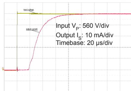
Figure 6: Typical step response (0 to 2800 V)
